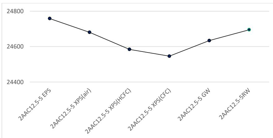
**TABLE 14.** TEC of AAC block and double wall with insulation materials.
