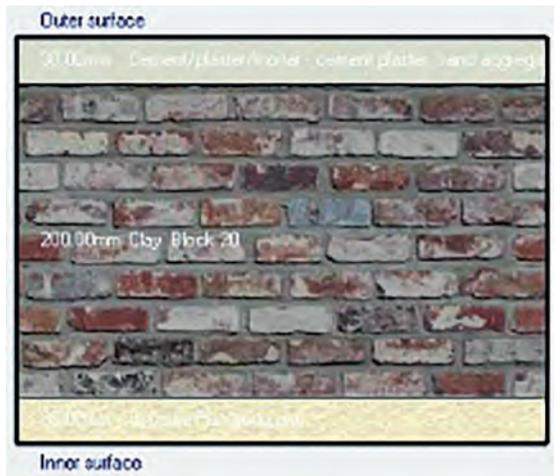
**FIGURE 7.** Wall Type 46 Layout, DesignBuilder.
