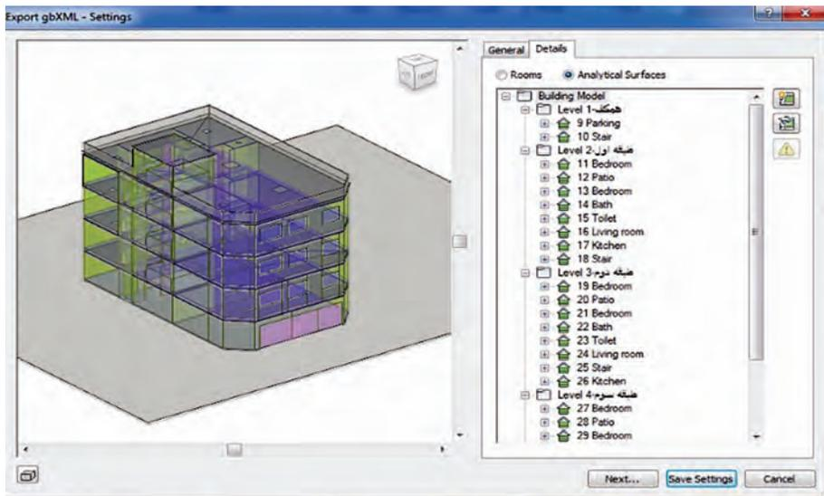
**FIGURE 5.** Model geometry layout in (DesignBuilder Software Ltd, 2019).
