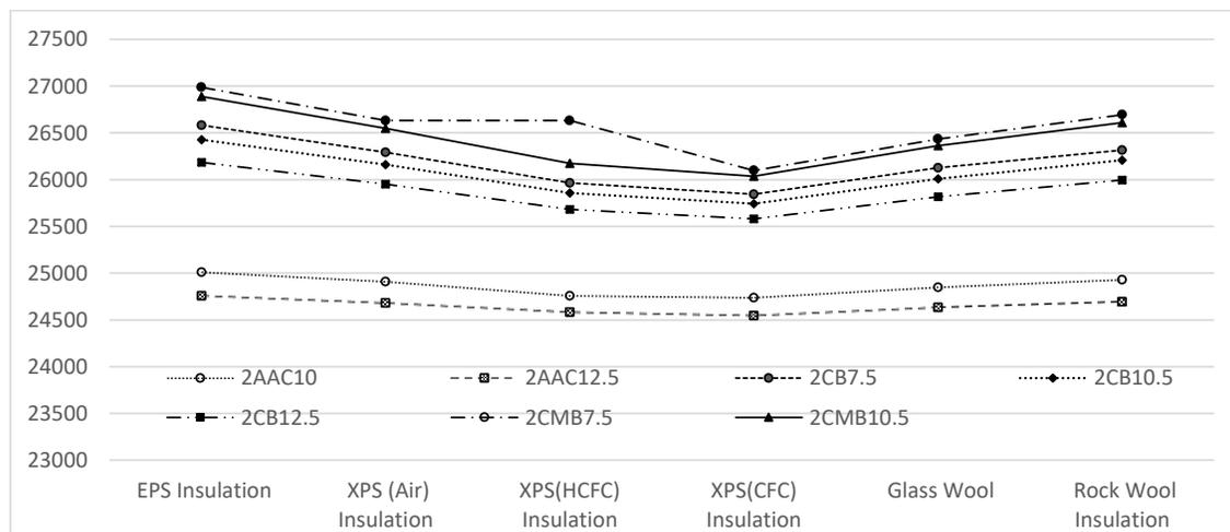
**FIGURE 9.** Total energy consumption of double external wall (kWh) based on insulation types.
