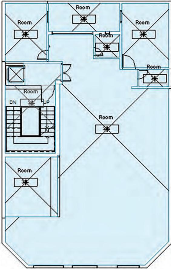
**FIGURE 4.** Exporting gbXML data file as an analytical model.
